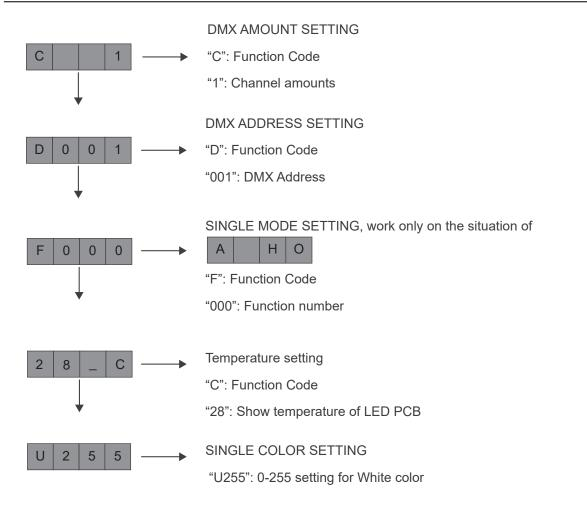
Press the "MODE" then press the "ENTER" to begin your setting. Press "UP" and "DOWN" to switch the modes with the shining Function Code. Be sure to press the "ENTER" button to save your changing, it won't be saved if the button has not been pressed. Moreover, the saving data still exists even after power off and then on.
