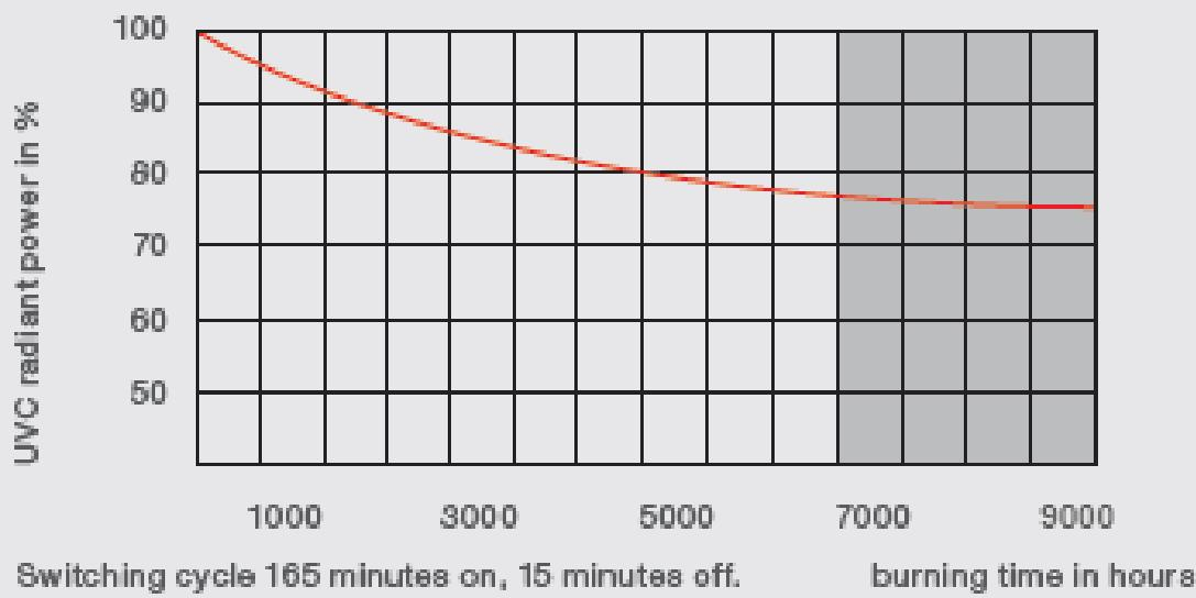
The lamps have a maximum life of 18,000 hours. To maximize the effectiveness of killing viruses and bacteria, we recommend replacing the lamps after 9,000 hours. The device signals the need to replace the lamp.
