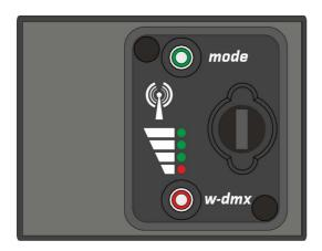
3. W-DMX is linked. DMX is missing on the Transmitter.
