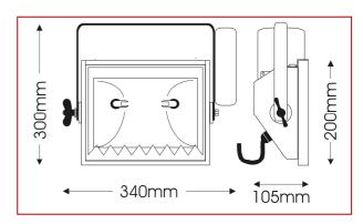
Stylish and high specification 70W asymmetrical discharge floodlight, ideal for usage in all those architectural, display and retail areas applications where a powerful yet low consumption and long lasting beam of light is required.
